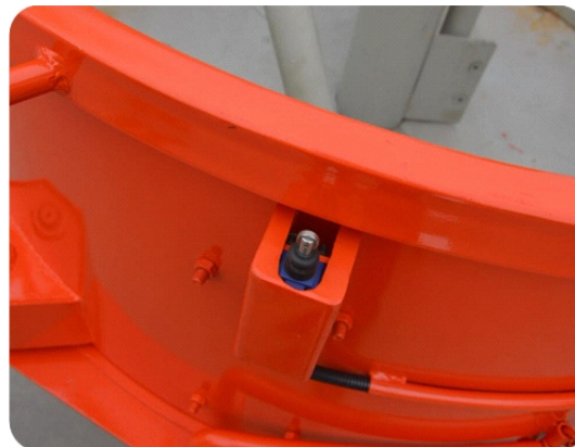
Limit switch for protecting operator
