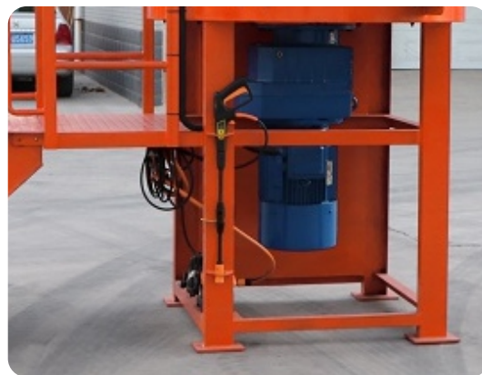
High pressure water washer device for GRM800
