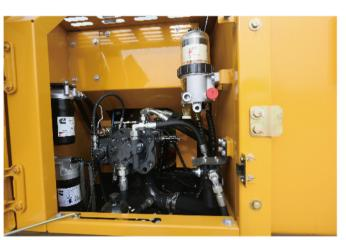
Fuel breather valve is standard equipped to keep the tank pressure stable, effectively filter dust, and ensure the oil quality. A wide range of after - sales service system and quick- response rescue mechanism can ensure that you use machine at ease.
