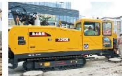
XZ450水平定向钻机在上海施工 XZ450 HDD working in Shanghai
