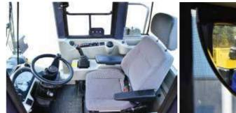
The full-coverage exquisite interior trim parts The super-large spherical rearview mirrors and the damping and noise reduction measures for the cab and engine hood reduce the noise by more than 6dB.
