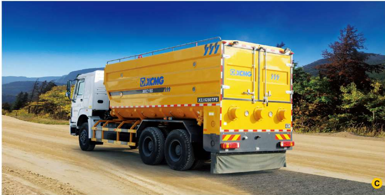
A、徐工沥青洒布车湖北施工 B、徐工JCM100W在G2513淮徐高速施工 C、徐工粉料洒布车安康施工 A、XCMG asphalt distributor in Hubei province B、XCMG JCM100W is under construction at Huaixu expressway G2513 C、XCMG powder distributor in Ankang
