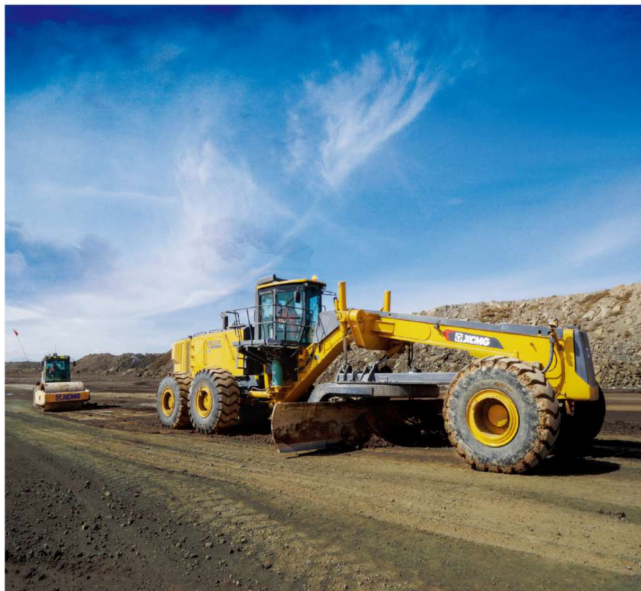
全球最大马力徐工GR5505平地机扛鼎大型露天煤矿 GR5505 grader with world's highest horse power performs in large open-pit coal mine
