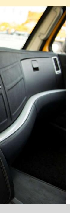
■ 防尘降噪高密封性两室,两室耳旁噪音从82.3分贝降低至78.3分贝,减少3分贝 Cabs with high air tightness, 3 dB(A) noise reduction in noise level at seated position from 82.3 dB(A) to 78.3 dB(A)
