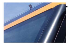
优化玻璃胶施工工艺,加 大涂胶面积,杜绝漏雨 Optimized construction technology of glass glue, increased glue coating area, no leakage of rain
