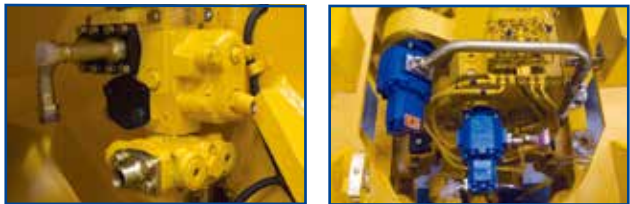
Flow amplifying valve Double-pump confluence
