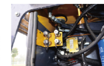
集中测压 Centralized pressure measurement
