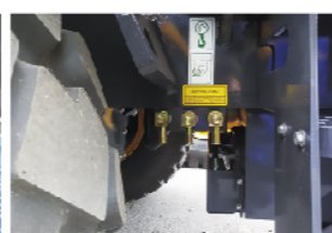
集中放水、放油 Concentrated water and oil release
