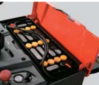
高性能的3PzS (4PzS) DIN标准电瓶, 适合长时间操作 The high-performance 3PzS (4PzS) DIN standard battery is suitable for long-time operations.
