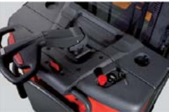
钥匙开关, 急停开关, 电量表 Key switch, emergency stop switch, and power level gauge
