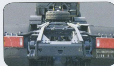
Frame: BeiBen unique frame, using the special material, punching in one time, high-loading ability
